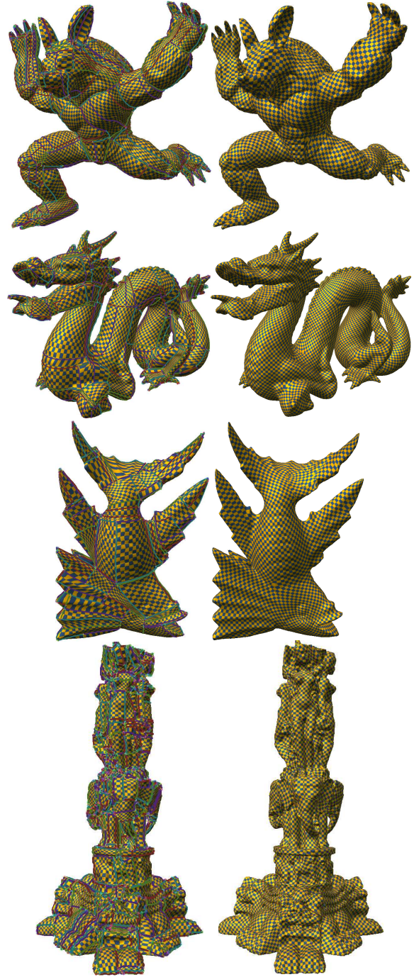
Figure 18: Comparison of the initial parametrizations computed from the consistent partitions (left) and the final parametrizations (right).
